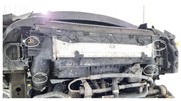
Remove the "under engine cover" 14x Hex 8mm screws.
