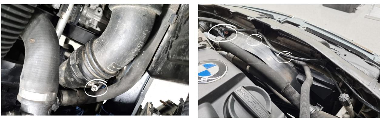
Remove the fresh air channel to the air filter box. 2x Torx T20 screws.
