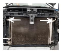
Place a steady support underneath the radiator pack.
