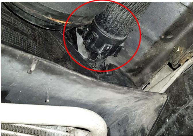
6. Remove the upper radiator hose (1x hose clamp & 1x metal clip) and also remove the bleeding hose (1x hose clamp & 1 plastic tab clips)
