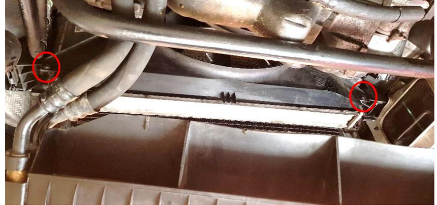
11. Remove the radiator fan. Loosen it with a 32mm open-end wrench. NOTE! It is left hand threaded. You need to keep the shaft fixed with a big flat end screw driver while loosening it. Lift the fan out of the car together with the fan cover.
