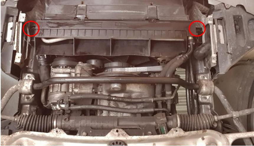
10. Remove all four radiator fan cover screws, Torx T25. Two in the top and two in the bottom.
