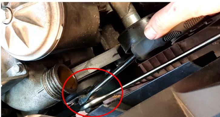
12. Remove 1x Torx T25 on the top left side of the radiator.
