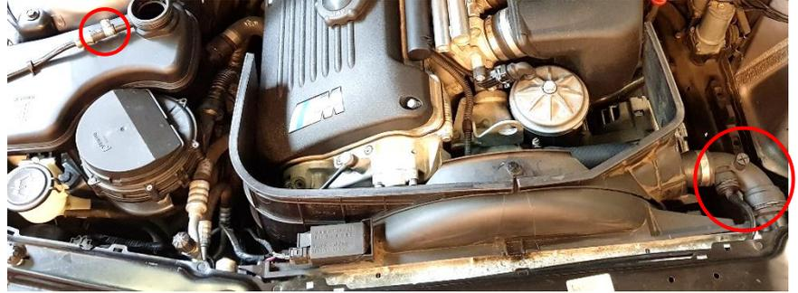
7. Remove the 3x plastic clips then remove the two radiator fan air guides.
