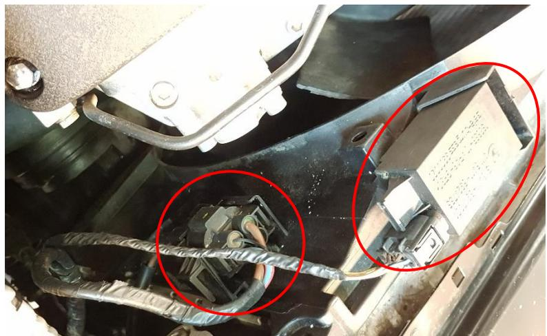
9. Remove the oil cooler from the radiator 2x Torx T25 screws. You don't need to disconnect the oil lines. Secure the oil cooler in a strap to the stabilizer sway bar.
