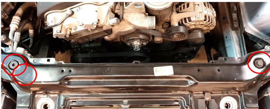
16. Install the included temperature sensor together with the included copper washer according to photo.
