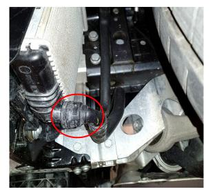
**10.** Remove the bottom screws, 2x Torx T30.
