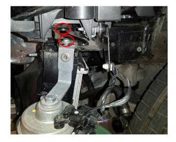
**11.** Remove the inner screws, 2x Torx T30. Reinstall these two screws once the radiator has been removed.
