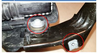
**13.** Install two of the rubber grommets and screw clip previously removed to the included bracket.
