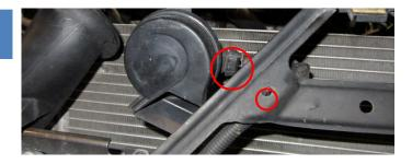
8. Remove the two Torx T25 screews that secures the air inlet pipe to the radiator support.
