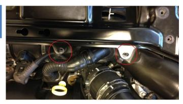
9. Remove the radiator support by removing 8pcs of 10mm (on facelift 6pcs) hex head screws on top of it and 2pcs of 10mm hex head screws in the bottom of the cross member.
