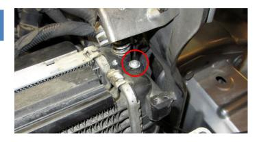
Remove the intercooler by lifting it up from the radiator slots and then carefully remove the intercooler downwards starting with the left hand side and then the rest of it according to picture.
