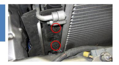
13. Lift the power steering cooling pipe up from its slots.
