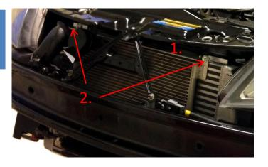
Remove the air guides on both sides of the intercooler by gentle pry out the tabs in the washer and then remove from intercooler pin. Remove air guides from intercooler.
