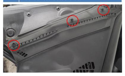
Remove this plastic clip with the help of a flathead screwdriver on both sides.
