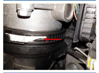
10. Use the included hose clamp to secure the do88 hose to the intercooler outlet pipe and intercooler.
