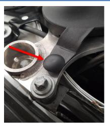
Remove 8x hex 13mm screws to the carbon fiber Strut brace, mounted across the engine.
