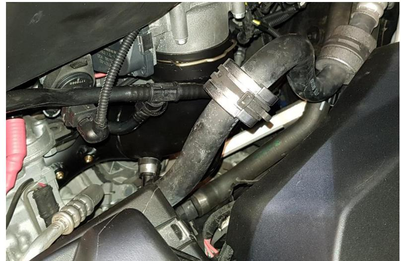
13. Push on the intercooler outlet hose onto the pressure pipe, do not tighten the hose clamp yet.
