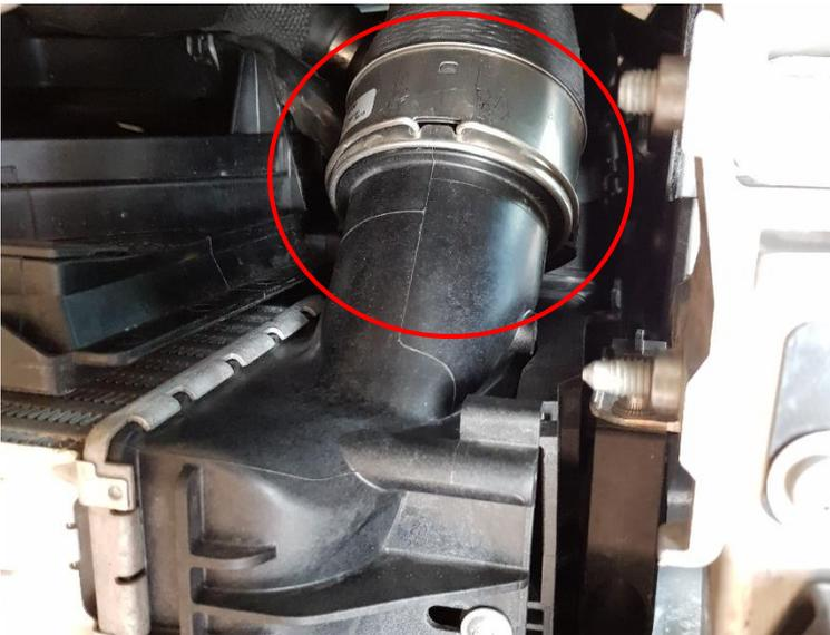
2. Pry the plastic tabs free on both sides for the front intercooler air guide.
