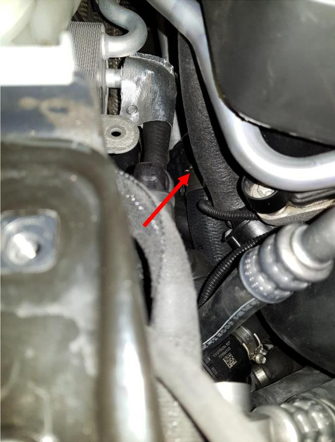
9. Install the sensor into the do88 intercooler pipe, fasten it with the included M6x14 screws.
