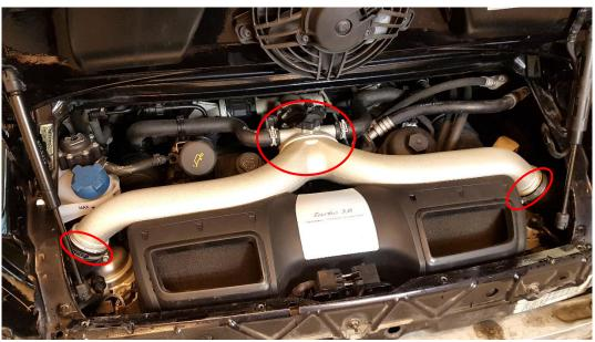
Remove the intercooler outlet hose (upper) from the intercoolers on both sides by prying out the quick coupling lock clips with a flat screwdriver about 10mm and then pull out the hose.
