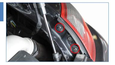
2. Remove 1pc Torx T30 plastic lock screws from the plastic clips on each side of the car located in the front of the space for the rear lights.
