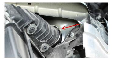
12. If you have bought the do88 Performance Y-pipe to fit together with the OEM intercooler setup, then you will need to reuse the OEM O-rings from the intercooler outlet hoses.
