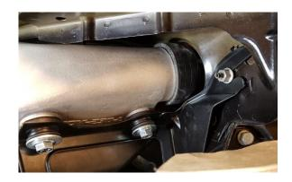
**15.** Re-install the air filter box and install the Y-pipe.
