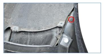
8. This step should be performed with the help of an assistant. Remove the bumper from the vehicle by carefully pulling it rearwards.
