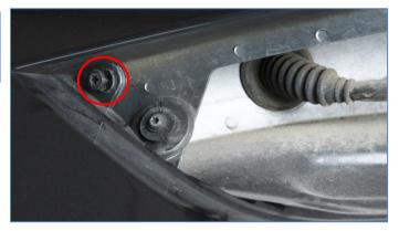
**3.** Remove 4pc Torx T30 screws located on the top of the rear bumper.
