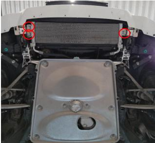
Loosen 2pcs 10mm hex screws on oil connectors and plug them with two included 16mm silicone caps to reduce oil leak. Now lift the oil cooler out of the car.
