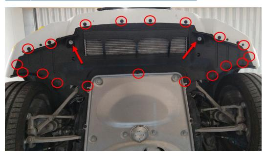
Remove 3pcs 13mm hex screws holding the oil cooler.
