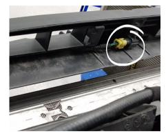
Disconnect the marked cable connector on the photo located on the backside of the radiator support. Loosen the cables from the radiator support.
