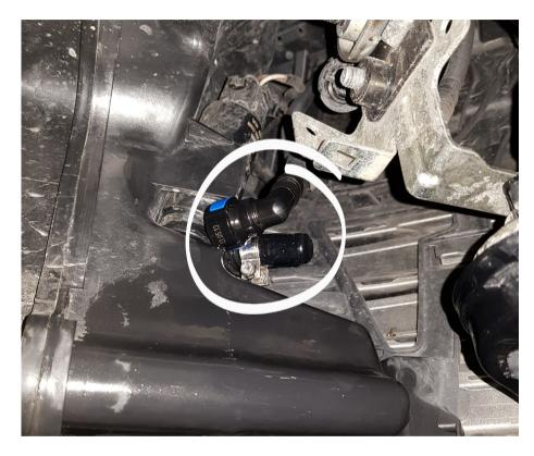
Cars equipped with headlight washers, disconnect the and use the included silicone cap to seal the connector.
