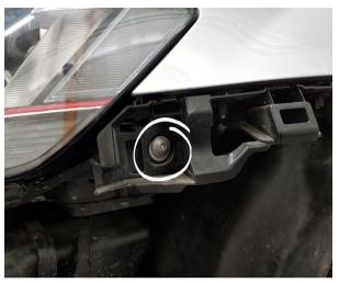
Step 12.2 Remove 1x Torx T30 screw. Do this on both sides of the headlights.
