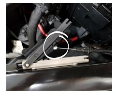
Unclip the hood cable joiner located over the left headlight.
