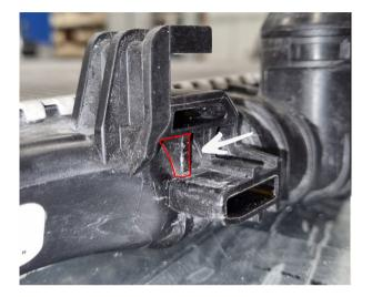
If your radiator does not fit in the lower slots of the do88 intercooler, you may need to trim the plastic tabs on the OEM radiator marked on the photo above.
