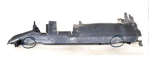
The left sides air guide needs to be slightly trimmed. Cut the plastic with a plier on the marked locations on the photo above.
