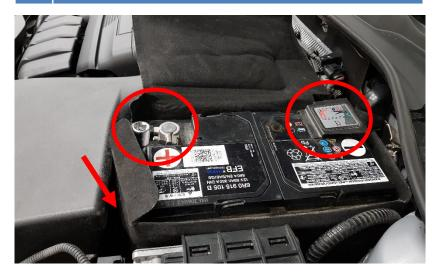
**3.** Loosen 1x Torx T30 screw at the pressure pipe bracket and 1x hose clamp on the turbo outlet. Also disconnect the small plastic box from it bracket on the battery tray.
