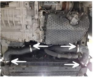
Step 17 Remove 2x Hex 10mm nuts marked on the photo. Step 18
