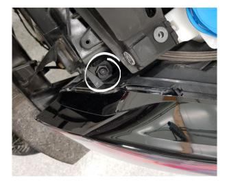
Step 12.1 Remove 1x Torx T30 screw. Do this on both sides of the headlights.
