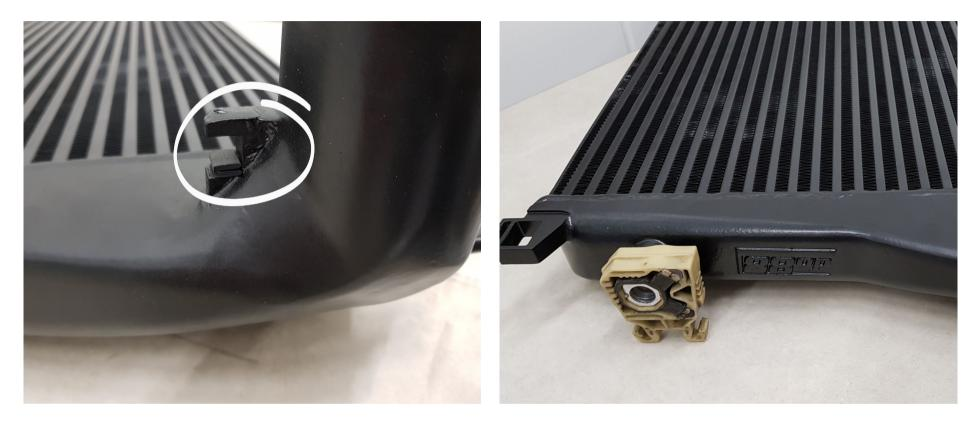
On both lower radiator brackets, put a piece of the included 4mm thick self adhesive rubber strip according to photo.
