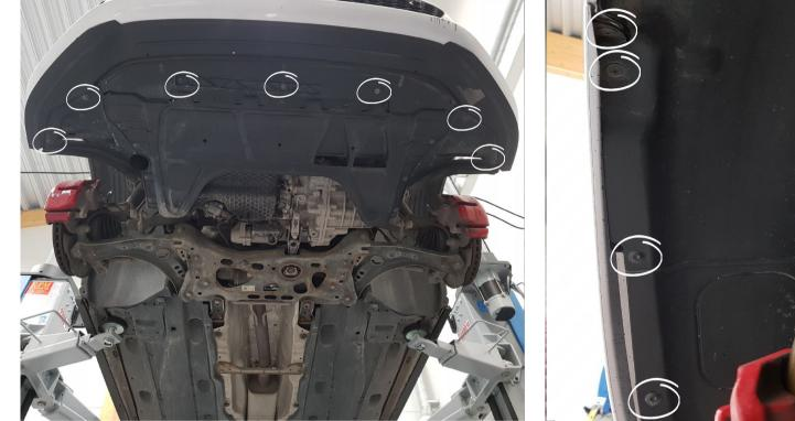
Remove 7x Torx for the plastic cover underneath the car.
