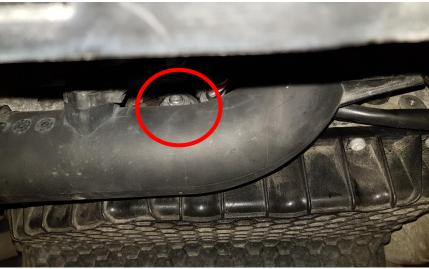
**12.** The do88 pipe comes with a 1/8 NPT meth injection connection. If you don't want to use this install the included blanking bung. <u>Screw it in carefully with some lubrication!</u>
