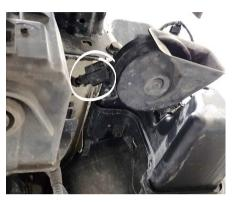
Step 16 Disconnect the cable connector for the horn.
