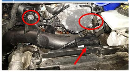
2. Remove the air filter box. Remove hose clamp, vacuum hose, SAI-connection (if your car has it). Then pull the air filter box upwards (it can sit quite hard in its rubber bushings).
