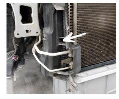
Remove the plastic air guides on both sides.
