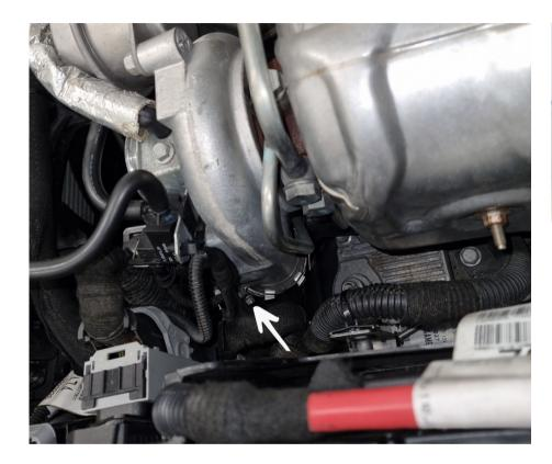
Remove 1x 7mm hose clamp located on the turbo outlet and remove the OEM intercooler hose from the car.
