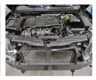
Remove Torx E12 screws on both sides of the car.(not located on the V6)
