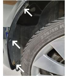
Step 2 Remove screws x3 inside the wheelhouse. Do this on both sides of the car.
