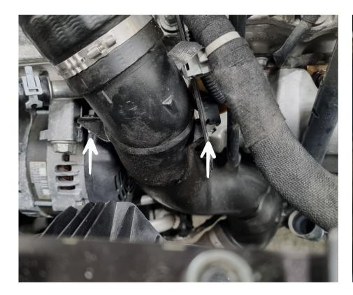
Remove 2x 10mm hex screws holding the OEM Intercooler pipe.
