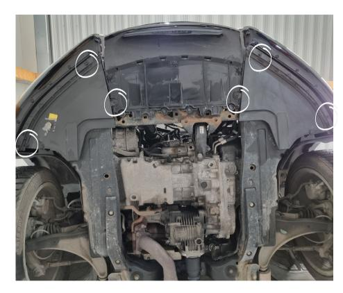
Raise your car up and remove 3x T25 screws on each side of the vehicle and remove the plastic covers. Do this to access and remove the hose clamps on the intercooler hoses on both sides of the car.
