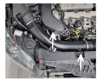
Step 3 Remove 2x 7mm hose clamps and 1x T25. Remove 1x T20 screw holding the sensor.
