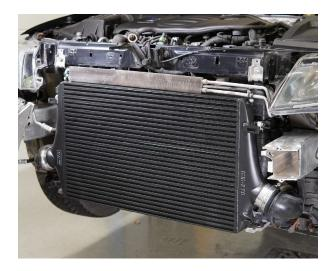
Install the power steering cooler and secure it with the 2pcs included rubber lined P-Clips and 2pcs M5x16mm screws, on top of intercooler.
