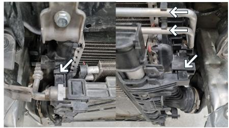
Remove screws x4 to remove plastic air guide.
