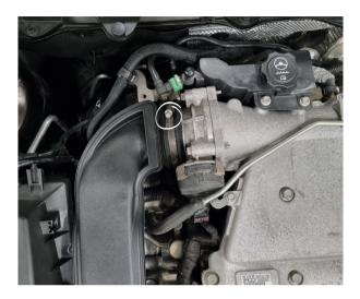
Step 5 Remove 1x hose clamp and remove the pipe from the car.
