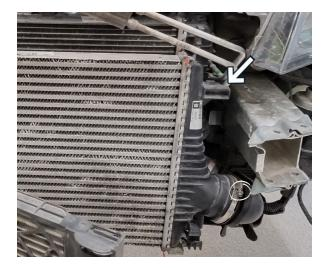
Remove clamps with a 6mm hex screwdriver and disconnect the intercooler pipes on both sides. Use a flathead screwdriver and gently push the plastic tabs to separate the intercooler from the radiator. Lift it out of the car.
